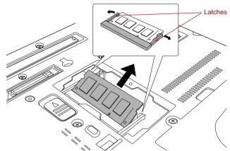
Figure 3-18 Removing the memory module
